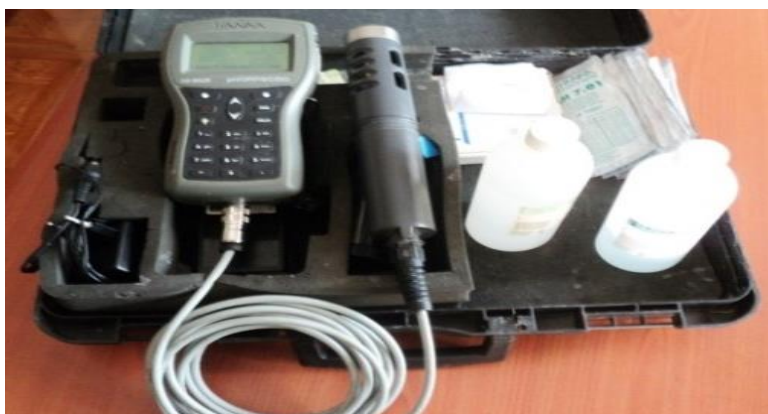
Figure 3-1: Multiparameter water quality meter (HANNA HI 9828) used to measure up to 13 different water parameters
