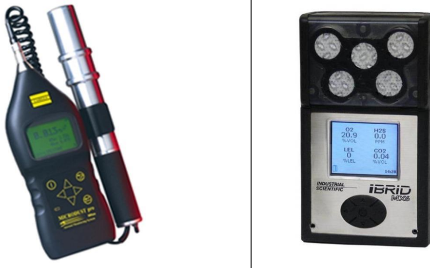
Figure 3-5: Digital CASSELLA microdust (L) and 6-gas MX6 iBrid™ meters(R) used to measure air quality
