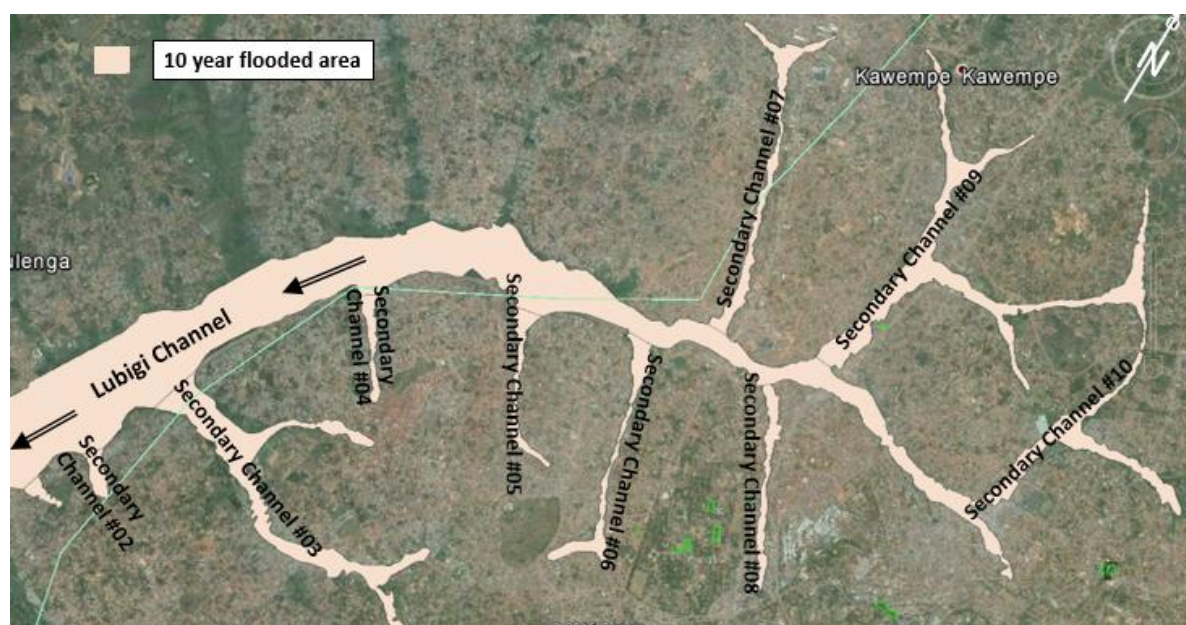
Figure 5-3: Lubigi Drainage System 10 year flood line generated in 2003 KDMP
