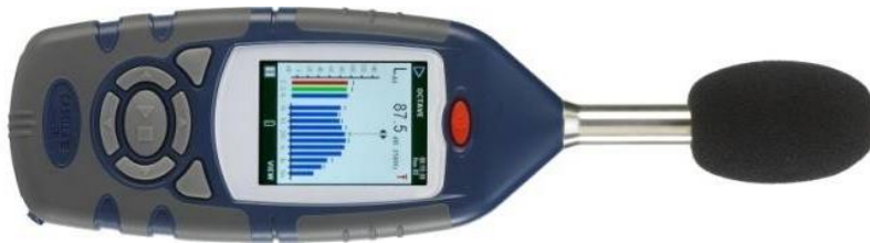
Figure 3-9: A CASELLA CEL-621C2/K1 Integrating 1/3 Octave Band Sound Level Meter (Class2) used for noise measurements
