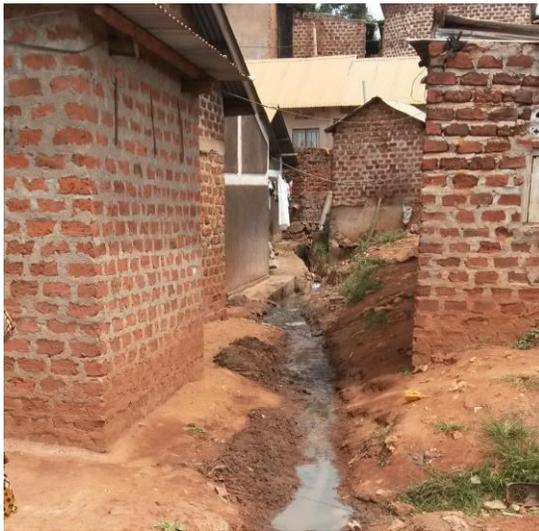
Figure 9: Toilet and Bathroom waste flowing into drains
